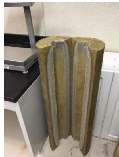
Stone wool after high temp exposure
