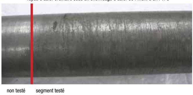
The corrosion science previously discussed and the lab testing are in agreement. Science shows why the corrosion can occur and why an effective moisture barrier on the interior surface of the metal jacketing should prevent this type of corrosion. The lab results are in complete agreement with the theory. The use of PSMB on metal jacketing protects all types of metal jacketing from this corrosion and protects the pipe under the insulation from this corrosion when the jacket is stainless steel.
